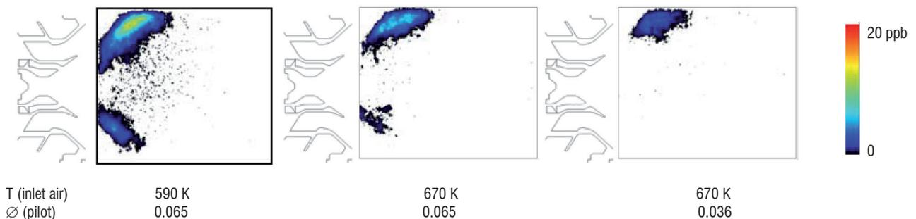
Figure 8 - Field of soot volume fraction obtained by LII downstream from a multi-point injector; pressure: 16.5 bar; global (stoichiometry): 0.36.
