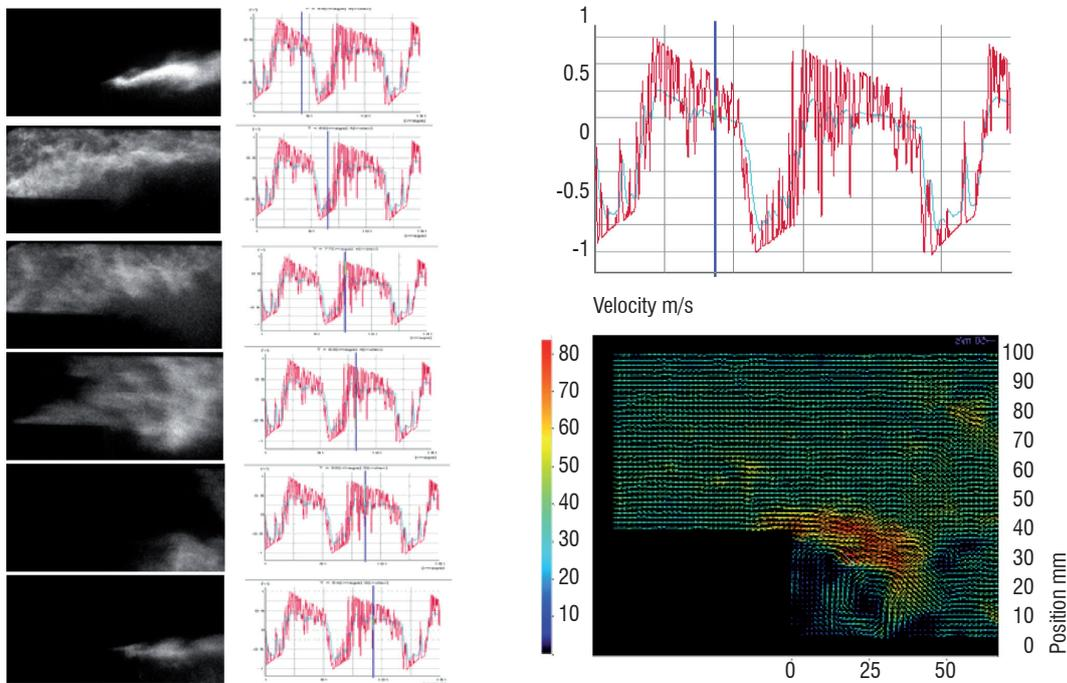
Figure 5 - Sequence of visualizations by OH\* chemiluminescence around the step corner and corresponding time (blue bar) during pressure evolution (left); evolution of the pressure measured on the upper wall displayed on a larger scale (upper right); Flow visualization around the step corner by PIV (lower right).
