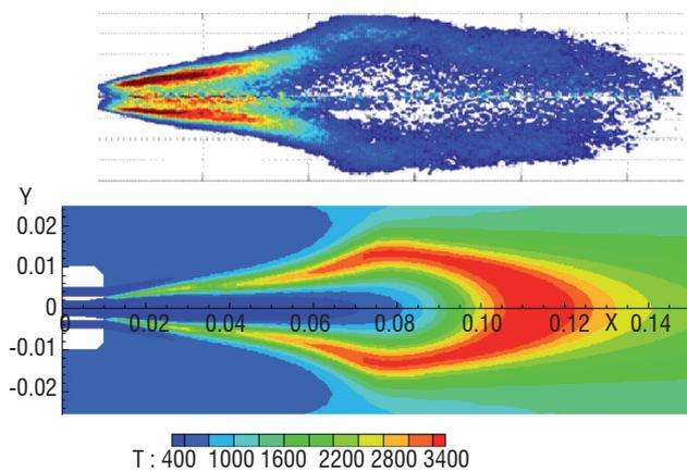
Figure 13 - Flow visualization by emission of  $\text{OH}^*$  obtained after Abel transform in transcritical conditions (top); temperature field obtained by RANS numerical simulation (bottom) in the same conditions.
