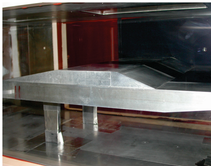
Figure 22 - Ramp model into the WT test section
