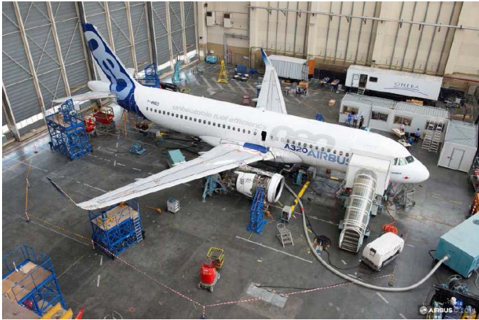
Figure 29 - GVT campaign on the A320 NEO PW MSN 6101 in Airbus facilities (Toulouse, France)
