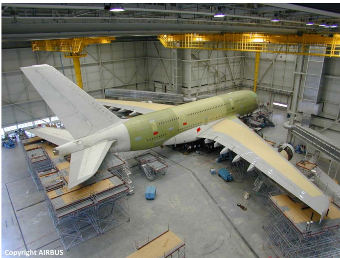
Figure 18 - General view of the A380 in the painting hall during the GVT
