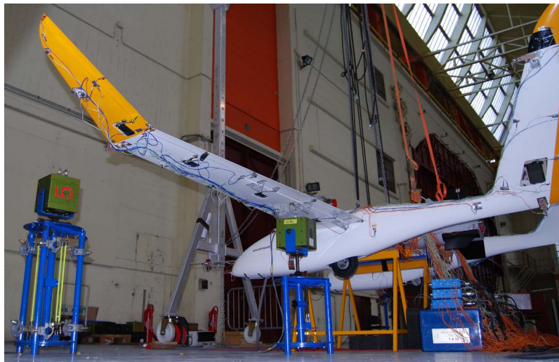
Figure 32 - EOLE UAV GVT (CNES, ONERA, Aviation Design, PERSEUS Student Project www.onera.fr/focus/eole )
