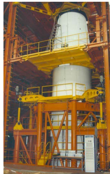
Figure 9 - GVT of Ariane IV sections in 1977
