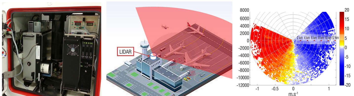
Figure 14 – left: ONERA high-power laser installed in the modified Windcube 200S ® ; middle: PPI scan for airport measurements; right: raw-wind data (radial wind speed) collected at Toulouse Blagnac airport. Data range up to 10 to 12 km
