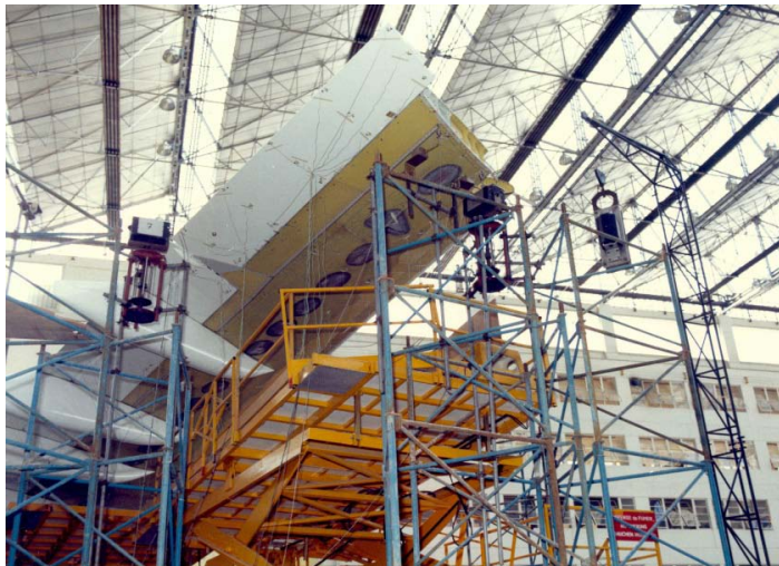
Figure 8 - 1 st Airbus (A300 B2) GVT in 1972
