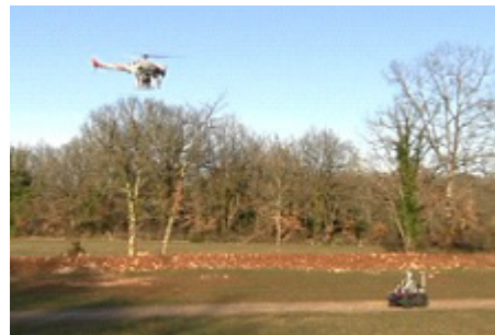
Figure 9 – Vision-based tracking of an autonomous mobile robot by an AirMax drone equipped with a monocular camera
