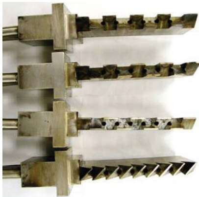
Figure 26 - JAXA strut injector concepts (with streamwise vortices)
