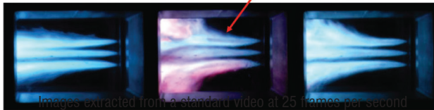
Figure 23 – HF burst observed in LOX/CH 4 operation (flow from right to left on the images of the video)
