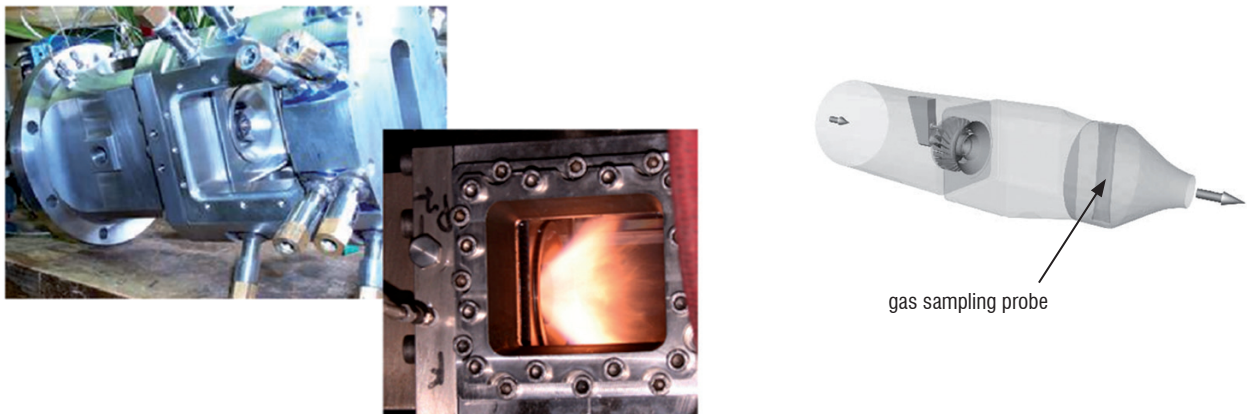
Figure 7 – Lateral view of the TLC combustor without and with combustion (left), schematic view of the TLC set-up with its downstream part including gas sampling probe and exit nozzle (right)
