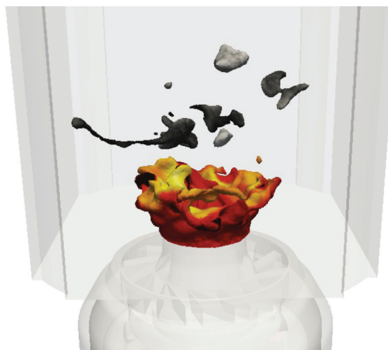
Figure 6 - LES of the DLR swirled turbulent flame [130]. Isocontour of temperature colored by the axial velocity (red-to-yellow) and soot ligaments colored by their number density (black-to-white).
