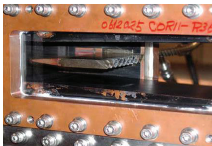
Figure 24 - View of a strut injector in the combustor
