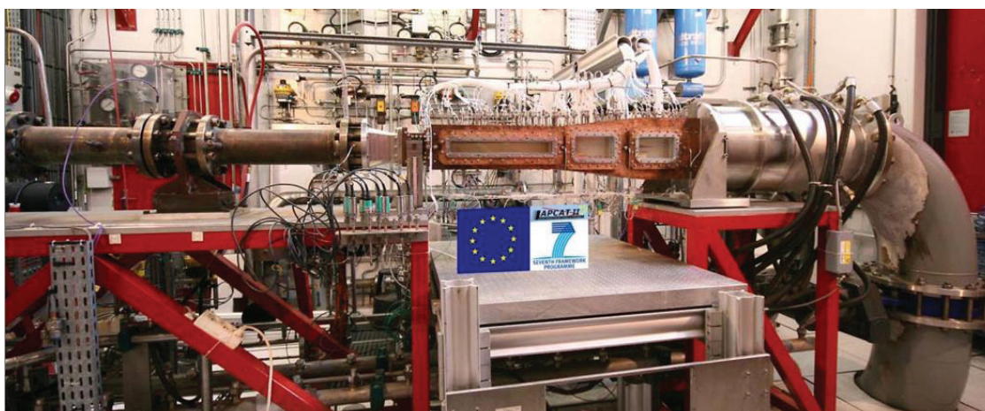
Figure 30 - Lapcat2 combustor installed in the Laerte facility
