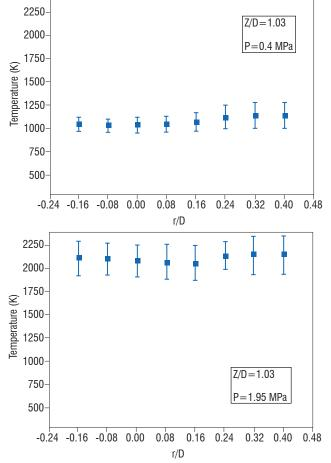
Figure 10 – Temperature profiles 65 mm downstream from the injector exit at 4 bar (left) and 19.5 bar (right) (abscissa: cross-coordinate r divided by D = 64 mm)
