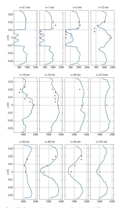
Figure 15 – Continuous lines: temperature profiles obtained by LES averaging; discrete points: CARS temperature measurements. All temperatures are plotted in K, x is the distance from the inlet section
