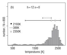
Figure 6 – Temperature statistics in the reference flame (a) at the stagnation point where the oxidation air jets meet and (b) low in the inner recirculation zone. The plots show mean and most probable temperatures and the width of the distribution, either as a range covering 90% of the instantaneous temperatures or as a width of a Gauss distribution where suited (dotted)
