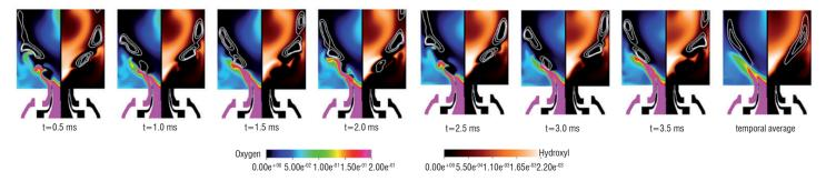
Figure 18 – Series of instantaneous and resulting time-averaged (right) distributions of calculated molecular oxygen (left hand side of the respective plot) and hydroxyl mass fractions (right hand side of the respective plot), as well as soot volume fraction isolines
