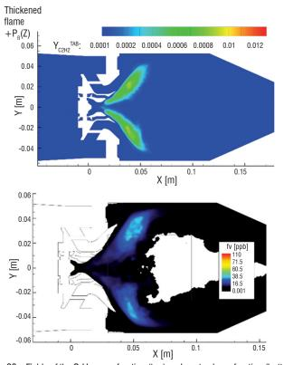
Figure 23 – Fields of the  $\rm C_2H_2$  mass fraction (top) and soot volume fraction (bottom) obtained numerically
