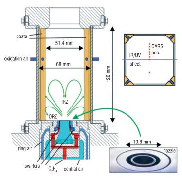
Figure 3 – Cross section of the DLR swirl burner operated with ethylene. The upper insert shows a horizontal cross-section at the height of the oxidation air inlets, as well as the locations of laser excitation for the diagnostics used
