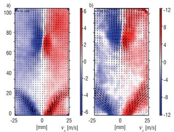
Figure 5 – Velocity fields of the non-reactive 3 bar case at  $\Phi$ =1.2 (left) and a leaner yet sooting and representative reactive case at  $\Phi$ =0.9 (right). Arrows show the in-plane velocity components, color represents the out-of-plane velocity
