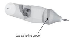
Figure 7 – Lateral view of the TLC combustor without and with combustion (left), schematic view of the TLC set-up with its downstream part including gas sampling probe and exit nozzle (right)
