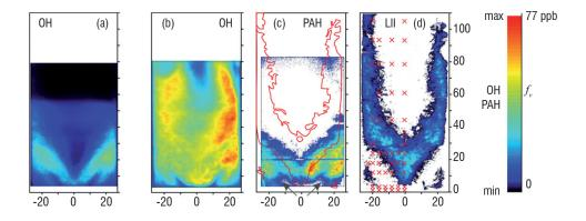
Figure 4 – Species distributions in reference flame (b) OH, (c) PAH, (d) soot. Without oxidation air injection (a) the OH distribution remains located at the bottom of the combustor; (c) also contains a contour of the soot distribution from (d), (d) shows labels where temperature statistics were measured by CARS
