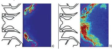
Figure 9 – Instantaneous LIF visualization of the fuel vapor (left, A), and of the OH radical (right, B); the same purple contour lines enclose the fuel vapor area on the left and right parts of the figure
