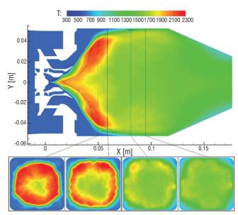
Figure 20 – Temperature field obtained numerically (temperatures in K); crosssection views are given for the four sections where CARS measurements have been performed
