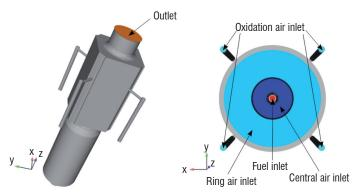
Figure 12 – The DLR burner: left, overall view of the burner and the plenum that supplies the injector; right, fluid supplies inside and beside the plenum upstream of the swirlers
