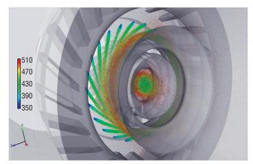
Figure 8 – Low NOx injector configuration; the colored part corresponds to simulated fuel droplets injected through the pilot (on the axis) and multi-hole devices (periphery); the color denotes the droplet surface temperature (scale in K)
