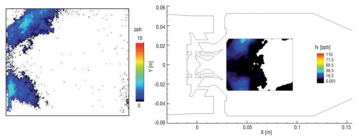
Figure 24 – Soot volume fraction obtained by LII (left) and by the calculation (right); the window shown in the calculated map corresponds to the measurement window displayed on the left
