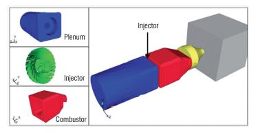
Figure 19 – Computation domain for the TLC calculation; plenum in blue, TAPS injector in green, combustor in red and choked nozzle in yellow
