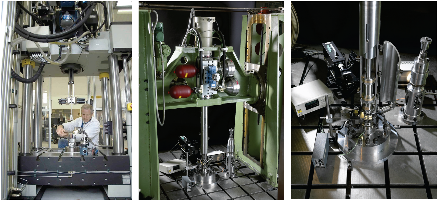
Figure 1 - INSTRON Hydraulic Jack (on the shelf, left), SCHENCK hydraulic machine (specific design, middle) and ONERA Titanium test rig developed for the SCHENCK facility (right)
