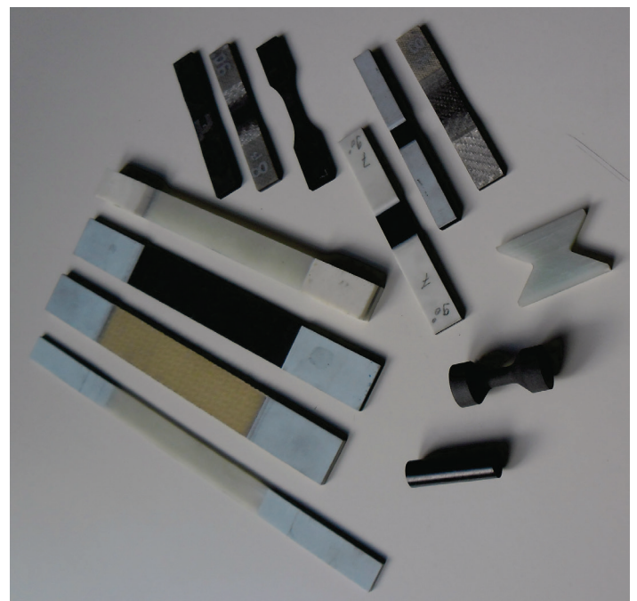
Figure 3 - Examples of specimen geometry for composite tension, compression and shear tests with hydraulic jacks
