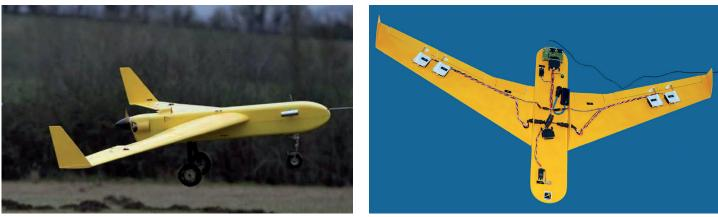
Figure 4 – UAV (left) and associated Iron Bird (right)
