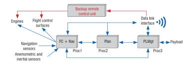
Figure 1 – Typical UAV 1<sup>st</sup>-generation architecture
