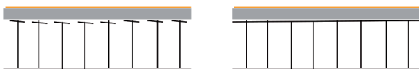
Figure 3 - Honeycomb sandwich panel, front side open (left) or closed (right), with absorption layer
