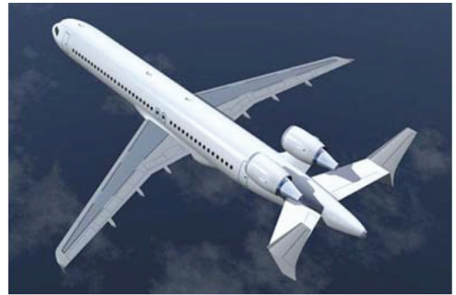
Figure 10 - Low Noise Aircraft based on the Rear Fuselage Nacelle concept (courtesy of Airbus)
