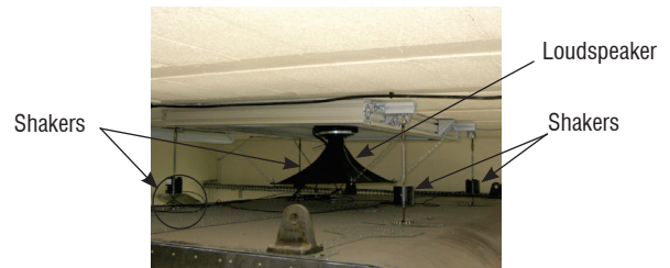
Figure 17 - Mechanical deck of an Onera cabin mock-up, with shakers and loudspeaker
