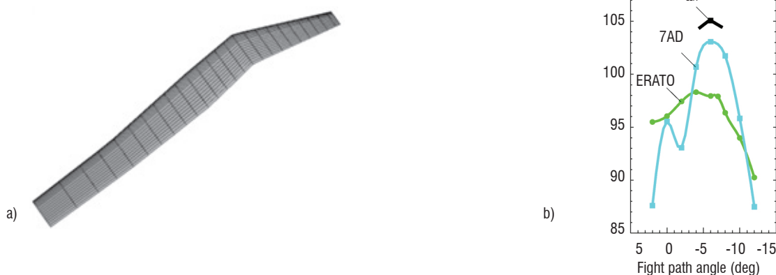
Figure 6 - a) ERATO blade shape. b) Noise reduction with ERATO blade measured at DNW (dBA) versus the descent angle at M_{\Omega R} = 0.617 .
