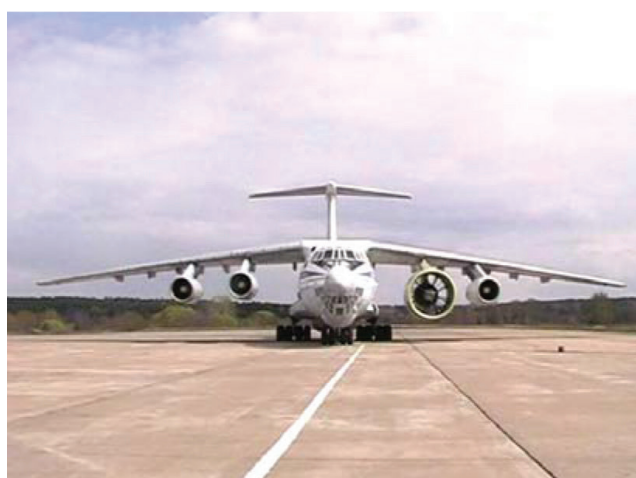
Figure 14 - The 1980 s Kuznetsov NK-93 on a flight test bed (left) and expected position of COBRA's deliveries on a noise roadmap (right)
