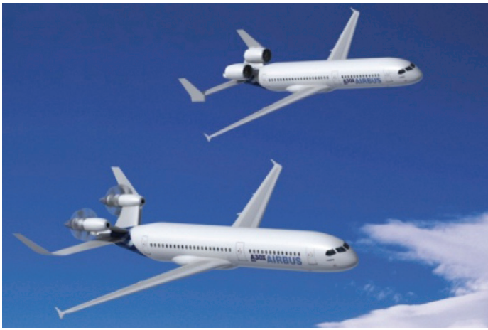
Figure 23 - Airbus views on a futuristic design for 2030 : rearward engines with or without Open Rotors (top) and embedded engines (bottom).
