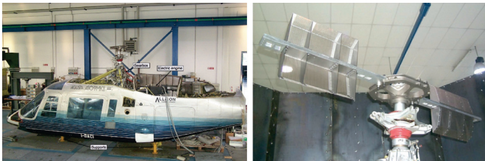
Figure 25 - Left: Helicopter mock-up, right: aerodynamic brake [21] (Politecnico di Milano)
