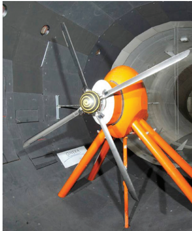
Figure 2 - a) Onera S1 Modane wind tunnel, b) Helicopter main rotor tests in the S1 Modane wind tunnel (active rotor)
