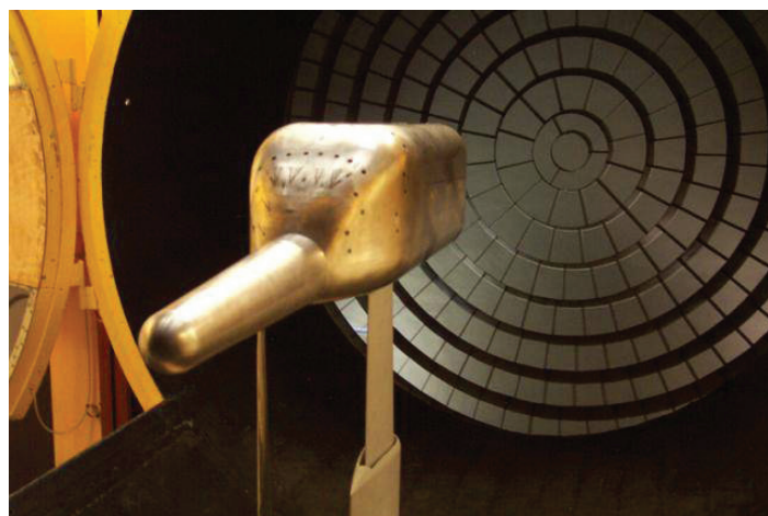
Figure 4 - ASF2 model mounted in Onera L1 wind-tunnel
