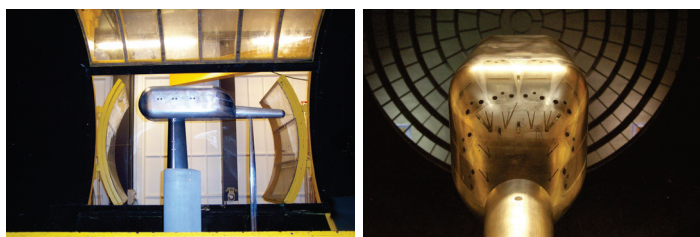
Figure 20 - GRC helicopter fuselage in the Onera L1 wind tunnel (left) and detailed view of the rear fuselage equipped with actuators (right)
