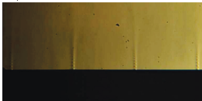
Figure 13 - Schlieren photography of the supersonic jets
