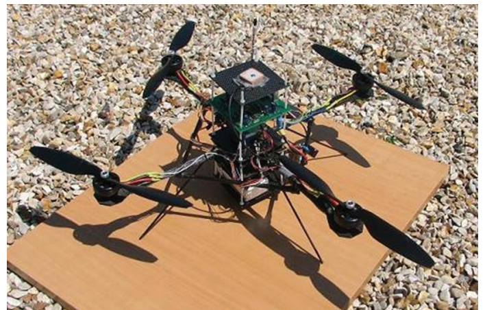
Figure 1 - Our home-built quadrotor : the "Quadricopter"
