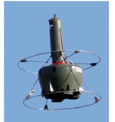
Figure 2 – Ducted-fan tail-sitter HoverEye of Bertin Technologies
